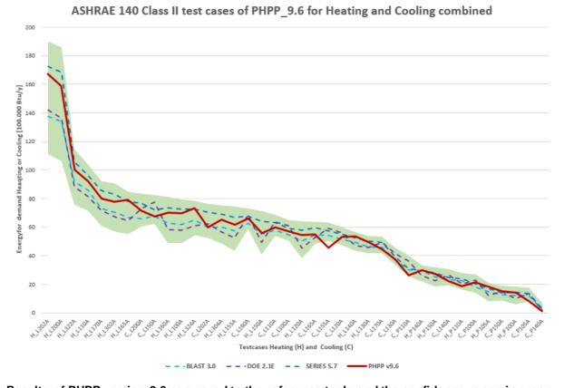
Results of PHPP version 9.6 compared to the reference tools and the confidence range in green, arranged according to magnitude of the results
