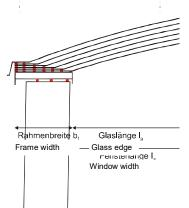
dix C. Deviation: profiles, for example for connecting window sills, belong to the frame. The actual glass insertion depth should be used.
